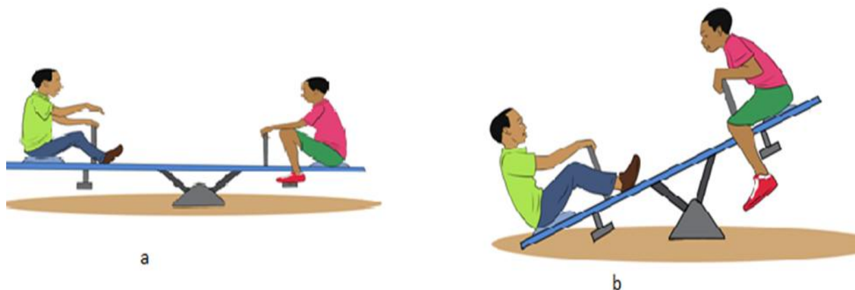
Figure 15.2: Students on in figure (a) represents a system in equilibrium. The equal and opposite forces on both ends of the seesaw are balancing. If, instead one force is greater in magnitude than the other, the combined force is greater than zero and is not in equilibrium as in figure (b)
